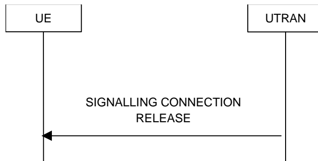
Figure 8.1.13-1: Signalling connection release procedure, normal case
