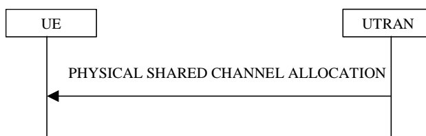
Figure 8.2.7-1: Physical Shared Channel Allocation
