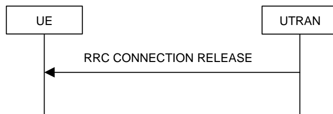
Figure 8.1.4-2: RRC Connection Release procedure on the CCCH
