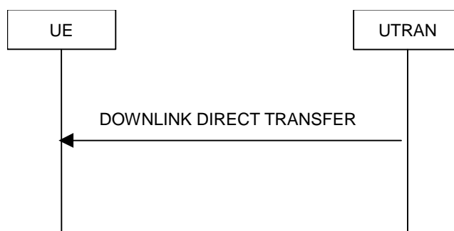
Figure 8.1.9-1: Downlink Direct transfer, normal flow
