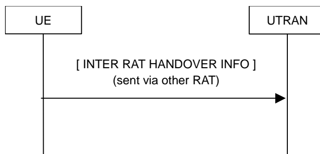
Figure 8.1.16-1: Inter RAT handover information transfer, normal flow
