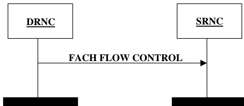
Figure 4A: FACH Flow Control procedure
