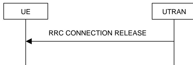
Figure 11: RRC Connection Release procedure on the CCCH
