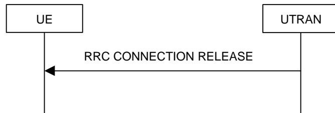
Figure 11: RRC Connection Release procedure on the CCCH
