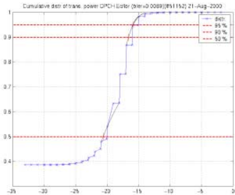
Figure 1549-12: Cumulative distribution of transmission power DPCH_{Ec} / I_{or} when compressed mode is on. TGL = 7 slots.
