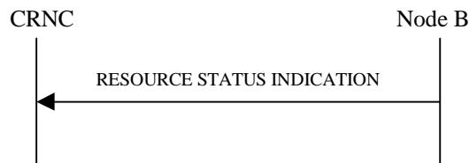
Figure 21: Resource Status Indication procedure: Successful Operation
