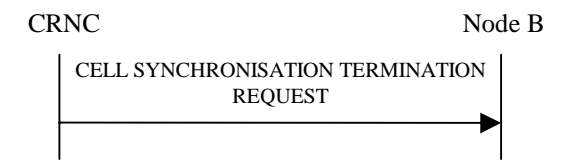
Figure 6: Cell Synchronisation Termination procedure: Successful Operation
