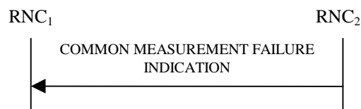
Figure x: Common Measurement Failure procedure: Successful Operation
