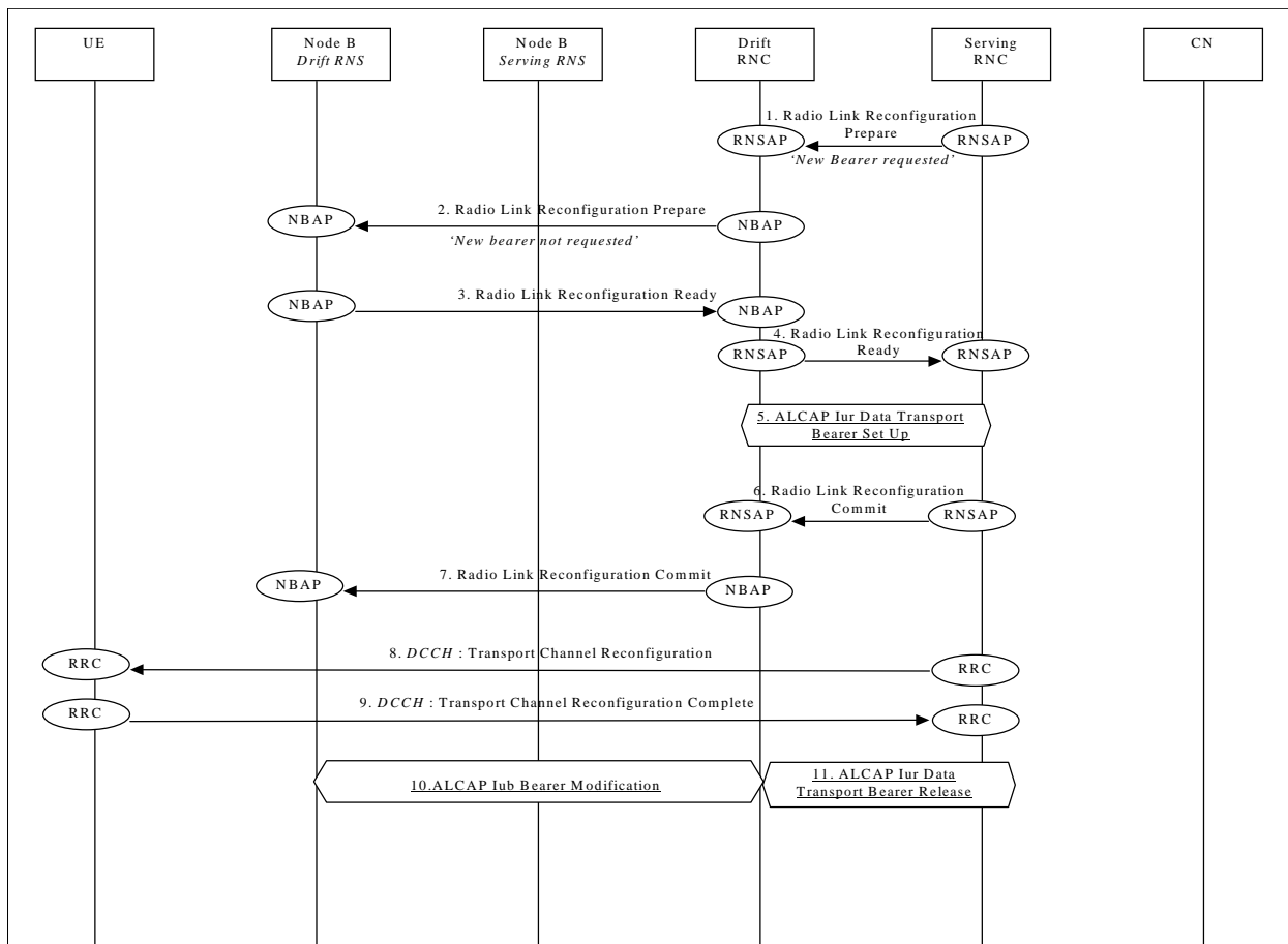
Figure 8: Synchronised Bandwidth Modification, Decrease (Interworking of Iub with the modification procedure and Release 99 Iur)
