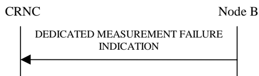
Figure 42: Dedicated Measurement Failure procedure: Successful Operation
