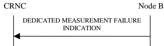
Figure 42: Dedicated Measurement Failure procedure: Successful Operation
