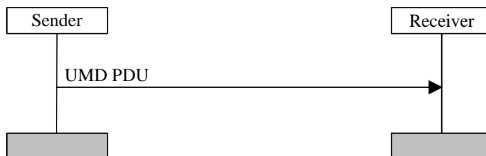
Figure 11.2: Unacknowledged mode data transfer procedure
