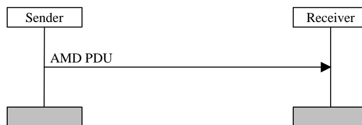
Figure 11.3: Acknowledged mode data transfer procedure
