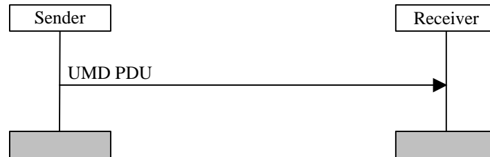
Figure 11.2: Unacknowledged mode data transfer procedure
