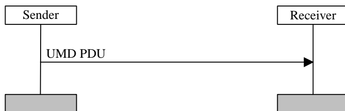
Figure 11.2: Unacknowledged mode data transfer procedure
