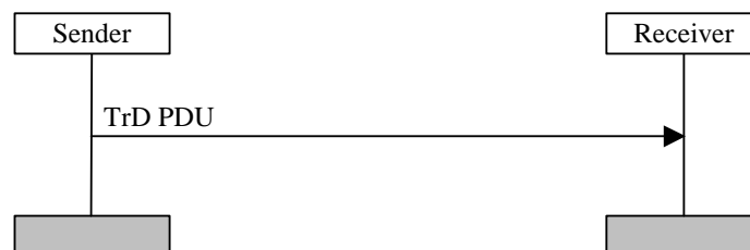
Figure 11.1: Transparent mode data transfer procedure
