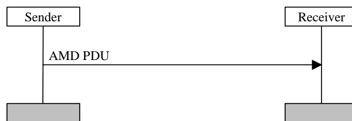
Figure 11.3: Acknowledged mode data transfer procedure
