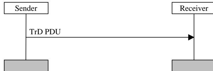
Figure 11.1: Transparent mode data transfer procedure
