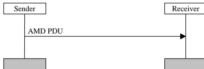
Figure 11.3: Acknowledged mode data transfer procedure
