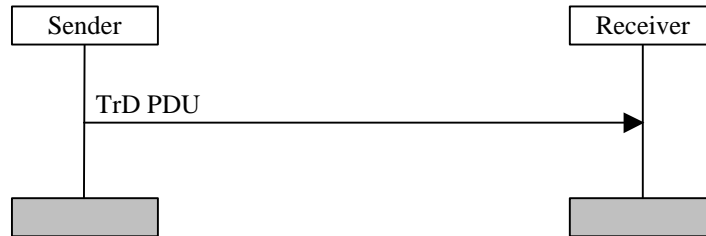
Figure 11.1: Transparent mode data transfer procedure
