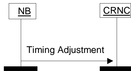
Figure 9: FACH, PCH and DSCH and [FDD – DSCH TFCI signalling] Timing Adjustment procedure
