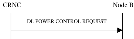
Figure 37: Downlink Power Control procedure: Successful Operation
