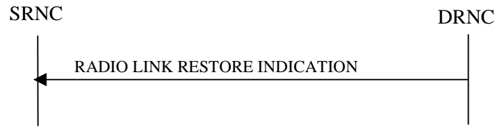
Figure 1: RL Restoration procedure, Successful Operation
