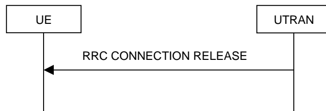
Figure 9: RRC Connection Release procedure on the CCCH
