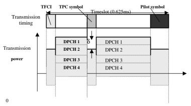
Figure 4-2012. Transmission power in multi-code transmission
