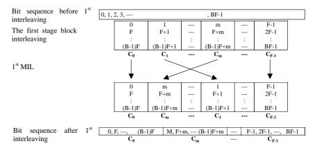
F: the number of radio frames corresponding to the transmission time interval B: the number of bits in a radio frame for the  $1^{\rm st}$  interleaving unit
