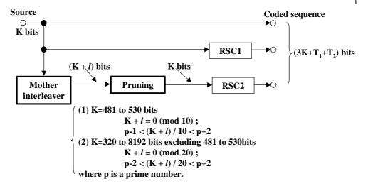
Figure 4-117. Overall 8 State PCCC Turbo Coding
