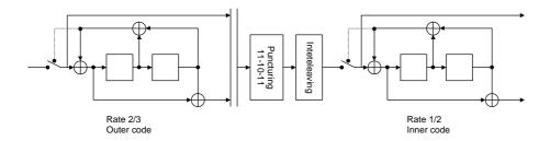
Figure 4-106. Structure of the 4 state SCCC encoder (dotted lines effective for trellis termination only)
