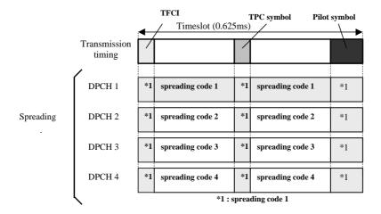
Figure 4-1811. Spreading code in multi-code transmission
