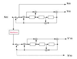
Figure 4-95. Structure of the 8 state PCCC encoder (dotted lines effective for trellis termination only)
