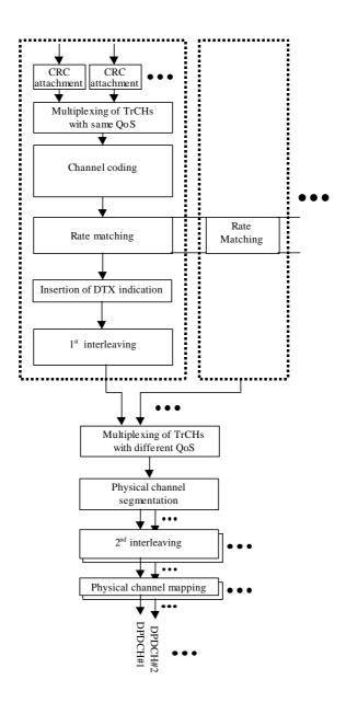
Figure 4-32. Transport channel multiplexing structure for downlink.
