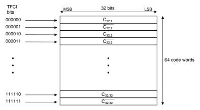
Figure 4-2414. Mapping of TFCI bits to biorthogonal code words.
