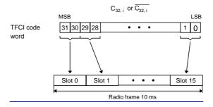
Figure 4-26.15. Time multiplexing of code words of (32, 6) code to the slots of the radio frame.
