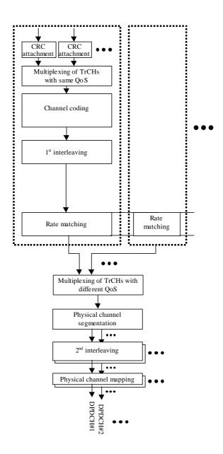
Figure 4-1. Transport channel multiplexing structure for uplink.
