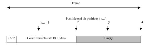
Figure A-1. An example of variable rate data format
