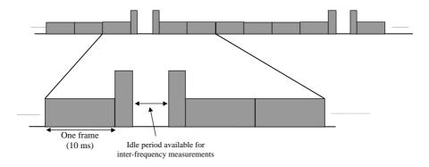
Figure 4-3017. Compressed mode transmission.
