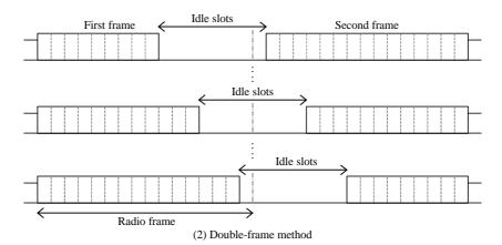
Figure 4-3821. Concept of adjustable transmission gap lengths position. < Editors note: Adjustment needed>
