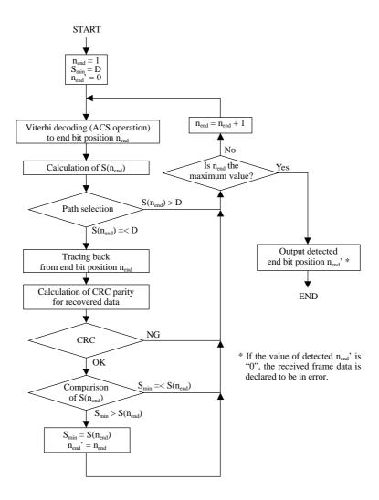
Figure A-2.Basic processing flow of blind rate detection
