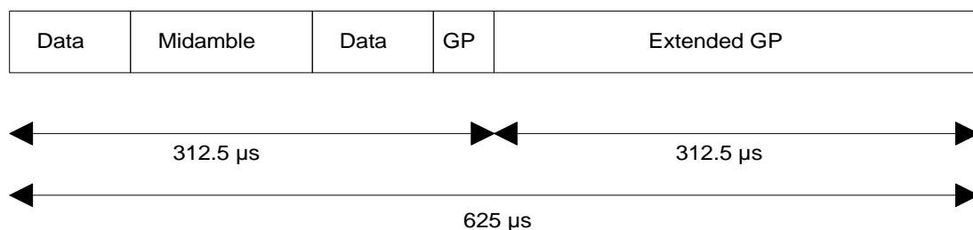
Figure 10 Access burst 1, GP denotes the guard period
