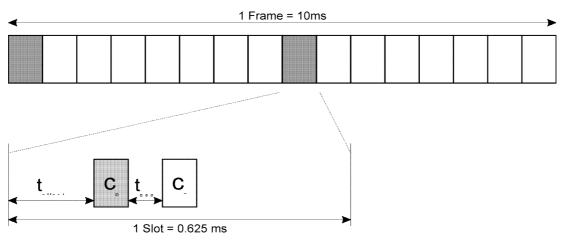
Figure 1: Structure of synchronisation channel (SCH)
