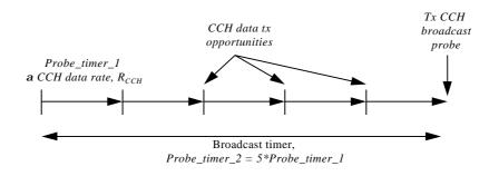
Maximum packet length =  $Probe\_timer\_l*R_{CCH}$
