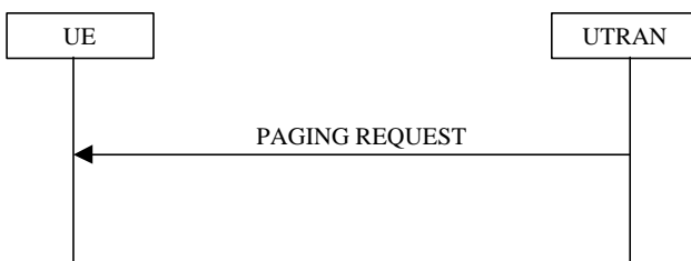
Figure 4) Paging request procedure
