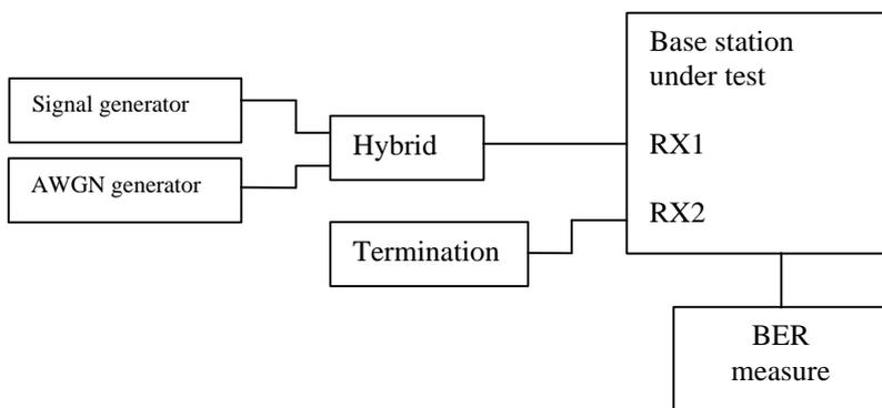
**Fig. 7.3-1** Measuring system set-up for dynamic range
