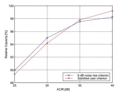
Figure 1. ACIR and capacity loss for UL 144 kbps data: intermediate case.
