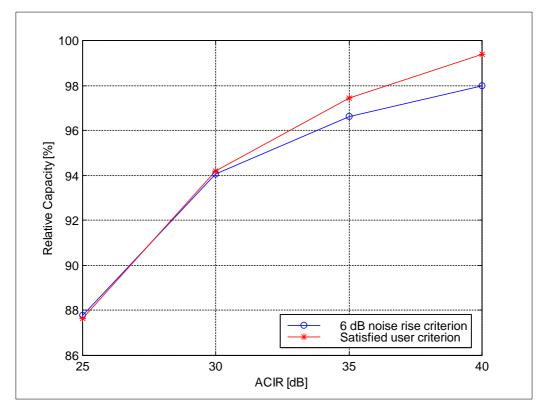
Figure 2. ACIR and capacity loss for UL 144 kbps data: worst case.
