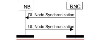
Figure X. "Channel" Node Synchronization procedure.
