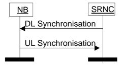
Figure 1. DCH Synchronisation procedure.
