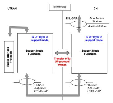
Figure 3: Iu UP protocol layer in support mode occurrence over lu interface
