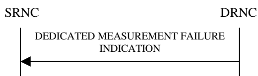
Figure 9-x: Measurement Termination Procedure initiated by DRNC
