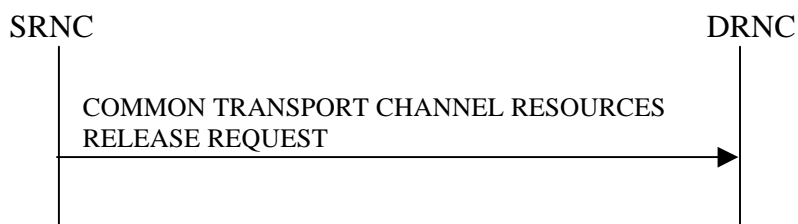
Figure 9-17: Common Transport Channel Release
