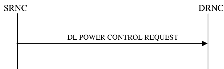
Figure 9-15: DL POWER CONTROL Procedure.
