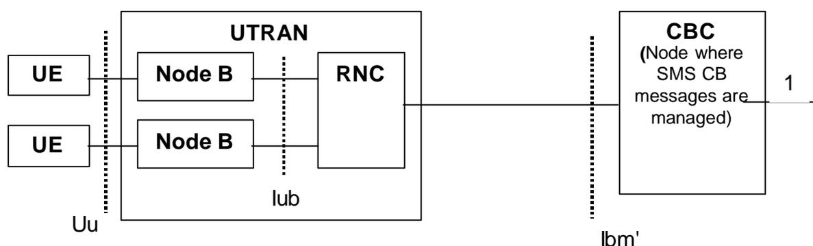
Figure 6.1: Architecture for SMS Cell Broadcast in UMTS for Case 1
