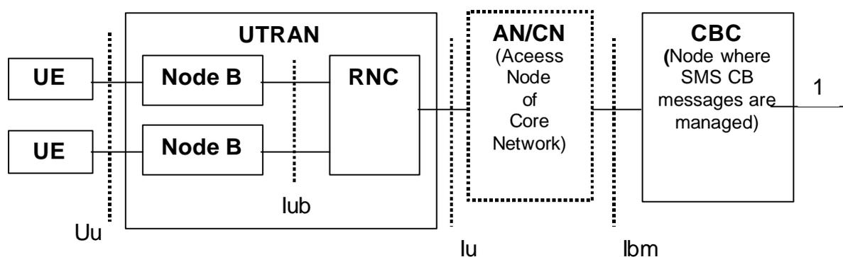
Figure 6.2: Architecture for SMS Cell Broadcast in UMTS for Case 2
