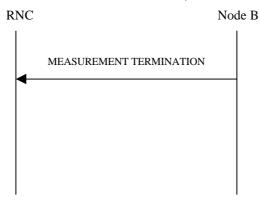
Measurement Termination Procedure initiated by NodeB
