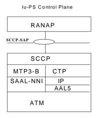
Figure 2 SAP between RANAP and its transport for the Iu -IP domain
