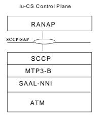
Figure 1 SAP between RANAP and its transport for Iu - CS Domain
