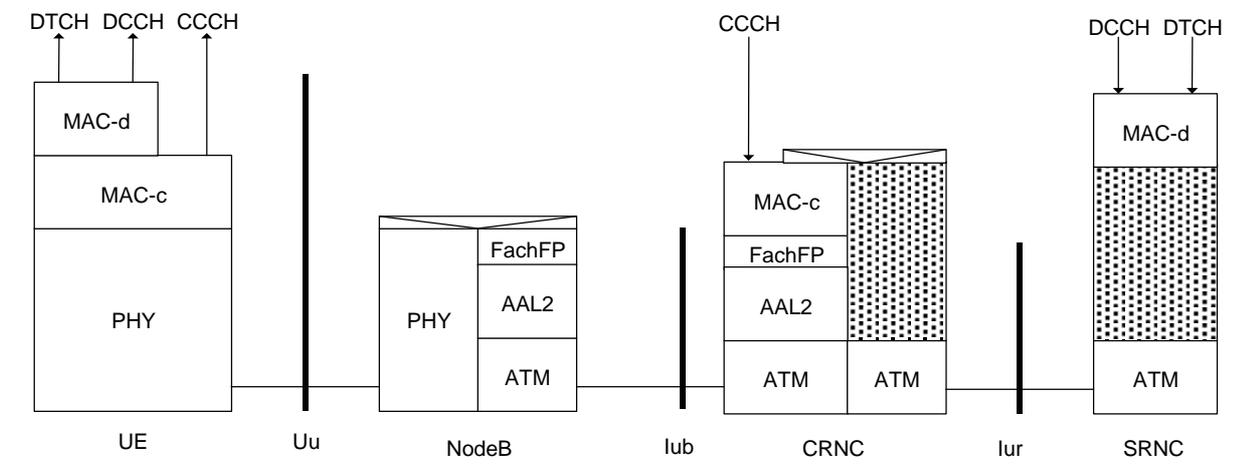
**Figure 23. FACH: Separate Controlling and Serving RNC**
