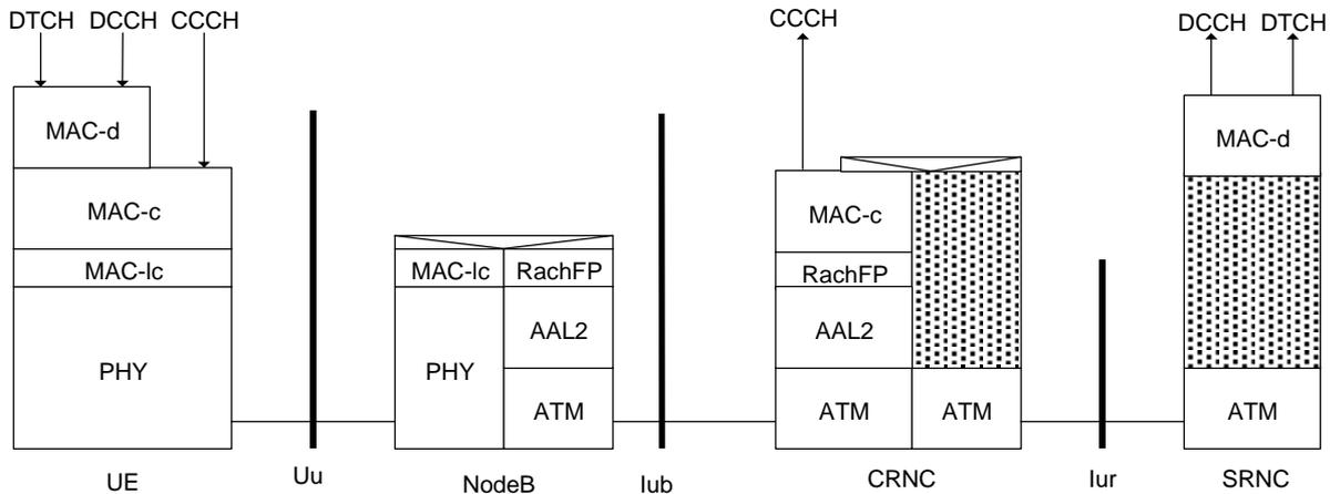
**Figure 21.** Figure 21 shows the protocol model for the RACH transport channel with separate Controlling and Serving RNC. In this case, Iur RACH Frame Protocol (DchFP) is used to interwork the Common MAC (MAC-c) at the Controlling RNC with the Dedicated MAC (MAC-d) at the Serving RNC (The exact Iur RACH Frame Protocol is FFS)
