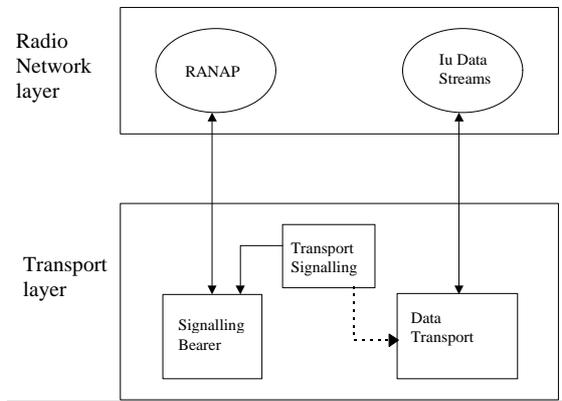
**Figure 15. Separation of RANAP and transport over Iu**
