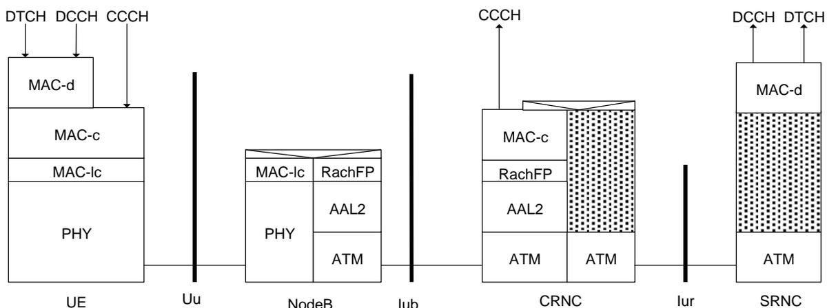
**Figure 21. RACH: Separate Controlling and Serving RNC**
