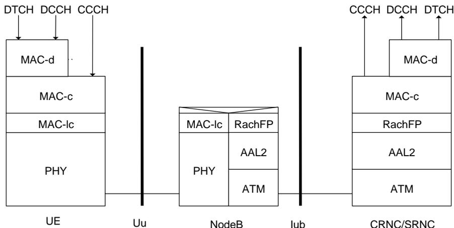
**Figure 20. RACH: Coincident Controlling and Serving RNC**
