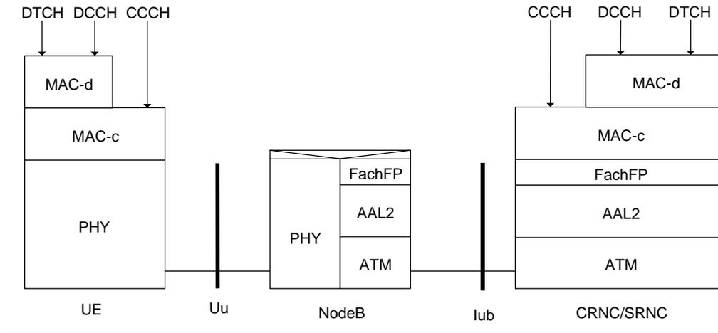
**Figure 22. FACH Co-incident Controlling and Serving RNC**
