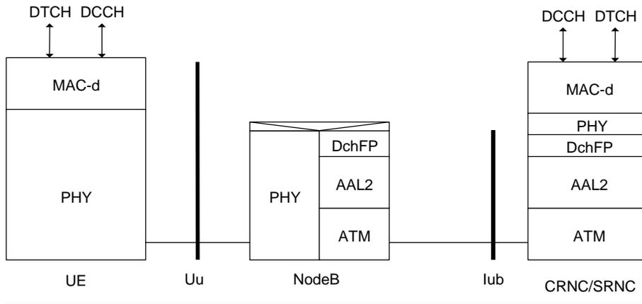
**Figure 24. DCH: Co-incident Controlling and Serving RNC**
