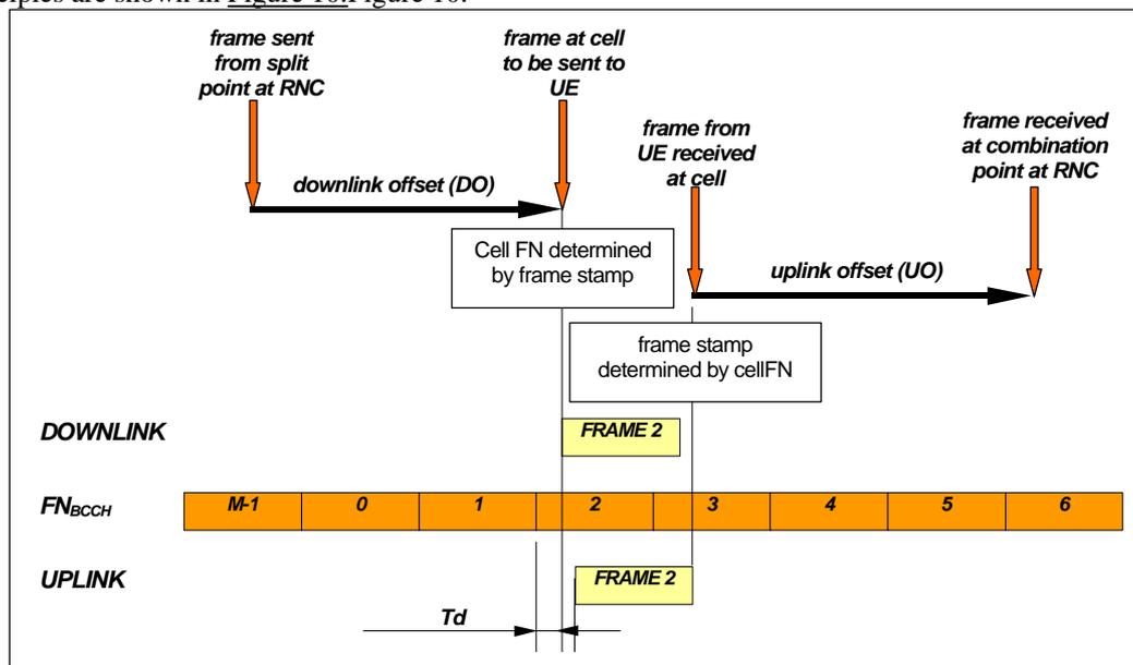
Figure 10. Frame stamping and uplink/downlink offsets handling
