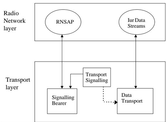
Figure 17. Separation of RNSAP and transport over Iur
