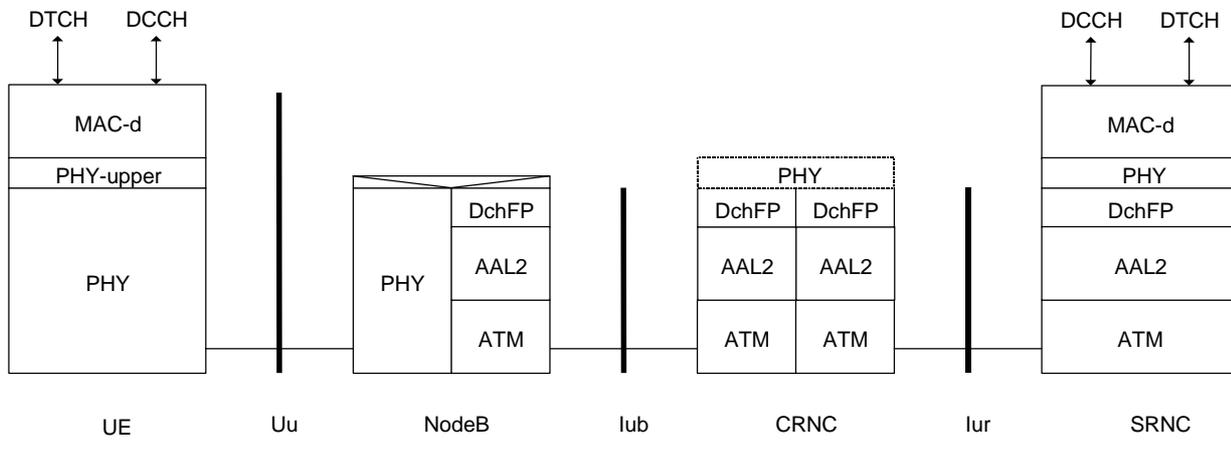
**Figure 25. DCH: Separate Controlling and Serving RNC**
