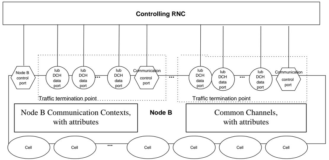
**Figure 18. Logical Model of Node B**
