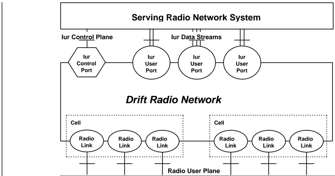
Figure 16. Drift RNS Logical Model
