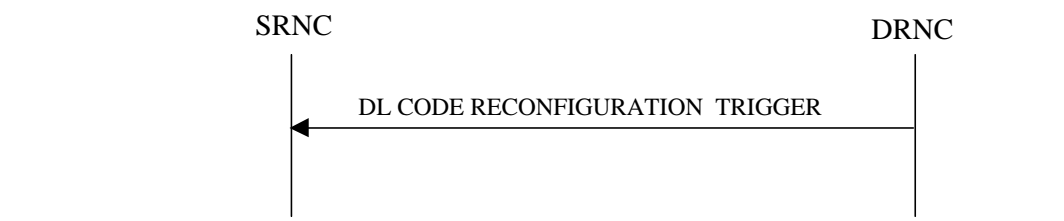
Figure 9-7. An example RNSAP message flow at I ur interface for DL Code Reconfiguration Trigger
