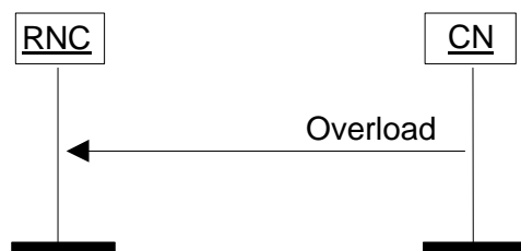
Figure 4. Overload at the CN.
