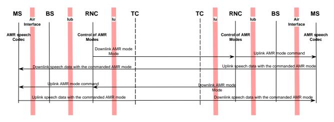
In this case, the local transcoder is not the final destination of the downlink codec mode command. The command must be transmitted (by some means) to the remote RNC to request the remote MS to use the best codec mode for the two involved systems. Note that in some cases, the remote network may be a GSM network also supporting in-band TFO or TrFO.
