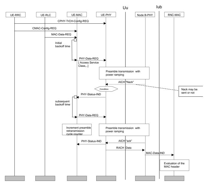
The RACH and AICH are configured once via a CPHY-TrCH-Config-REQ primitive. This primitive is issued only for initial configuration or when a parameter shall be changed, not for every RACH transmission.
