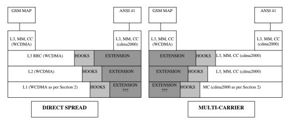
Figure 1. Protocol Structure for Implementing the Modular Concept
