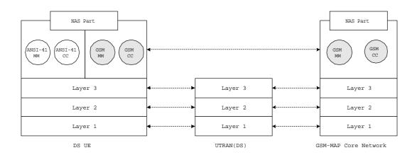
(b) Protocol Structure of DS UE for connecting GSM-MAP CN
