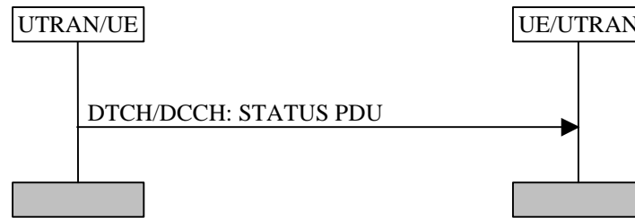
Figure 11-5. STATUS PDU transfer procedure.
