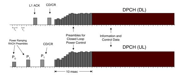
FIG 1. Common Packet Channel (CPCH) Timing Diagram with its Associated Downlink Dedicated Physical Channel.
