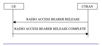
Figure 101010) Radio Access Bearer Release Procedure
