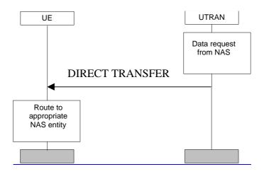
Figure 282828) Direct Transfer procedure in downlink
