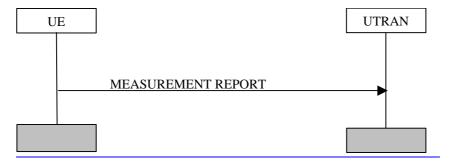
Figure 242424) Measurement Report procedure
