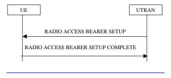
Figure 999) Radio Access Bearer Establishment Procedure
