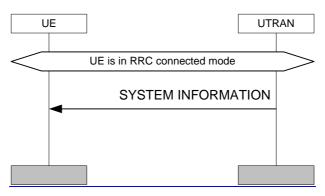
Figure 262626) Sending of system information to UE in RRC connected mode
