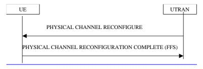
Figure 141414) Physical Channel Reconfiguration procedure
