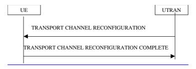
Figure 121212) Procedure for transport channel reconfiguration
