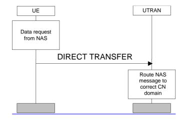
Figure 272727) Direct Transfer procedure in uplink
