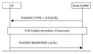
Figure 222222) UTRAN originated paging procedure in connected mode
