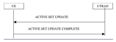
Figure 151515) Procedure for modifying the active set when in soft hand-over
