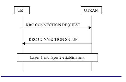
Figure 666) Procedure for RRC connection establishment
