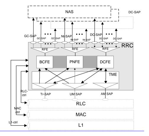
Figure 1) UE side model of RRC
