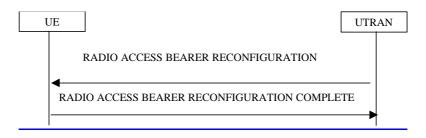
Figure 111111) Radio Access Bearer and signalling link Reconfiguration Procedure
