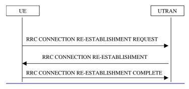
Figure 888) RRC Connection re-establishment
