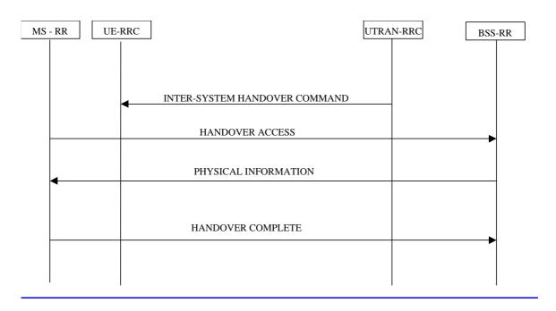
Figure 181818) Inter system hard hand-off (UTRAN to GSM/BSS), PSTN/ISDN services
