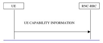
Figure 252525) Procedure for transmission of UE capability information
