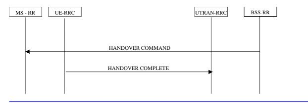
Figure 171717) Procedure for Inter-system hard hand-over - GSM to UTRAN
