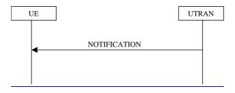
Figure 555) Notification procedure
