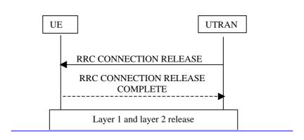
Figure 777) RRC Connection release procedure
