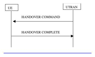
Figure <u>161616</u>) Inter-frequency hard handover
