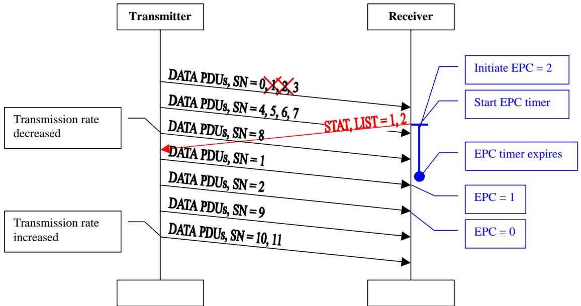
Figure 1. The estimated PDU counter and EPC timer.
