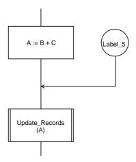
Figure 9: Example of poor use of a connector symbol
