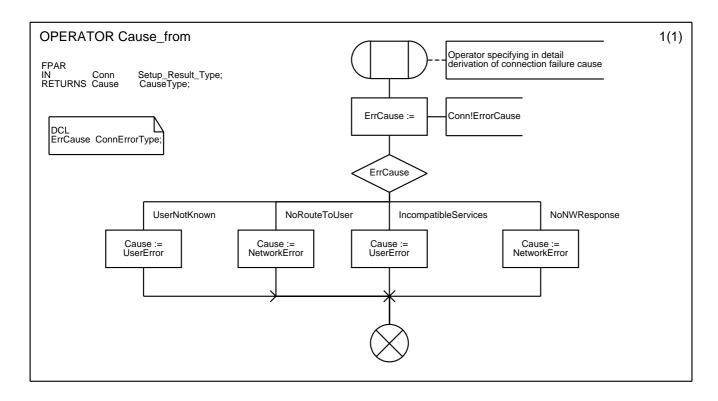
Figure 28: Example of detailed operator diagram
