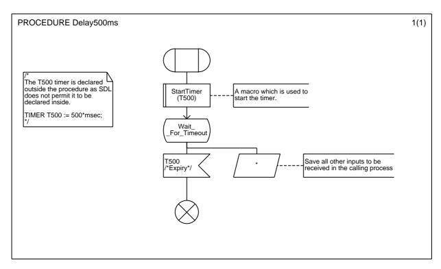
Figure 22: Example of a procedure containing a state
