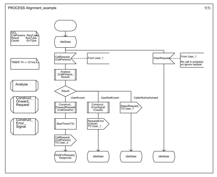
Figure 12: Example showing the alignment of NEXTSTATE symbols
