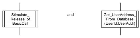
Note that in converting such text into a procedure call it may be necessary to add parameters to fully formalize the interface to the procedure.
