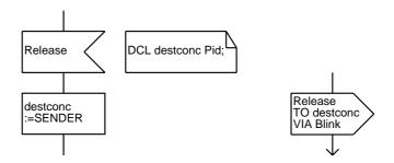
Figure 52: Replying to a sender.
