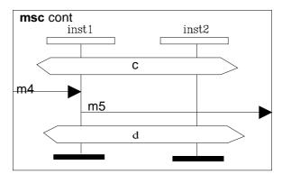
Figure 78: MSC with global initial and final conditions
