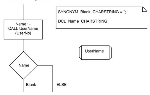
Figure 40: Decision based on a variable assigned from a value procedure
