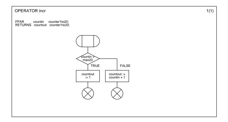
Figure 25: Operator diagram for the increment operator
