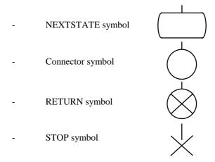
In the example shown in Figure 12, the processing on the page can end in a number of different states. The alignment of all of the associated NEXTSTATE symbols at the bottom of the page makes it clear what all of these possibilities are.
