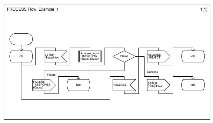
Figure 2: Example of poor layout of legal SDL
