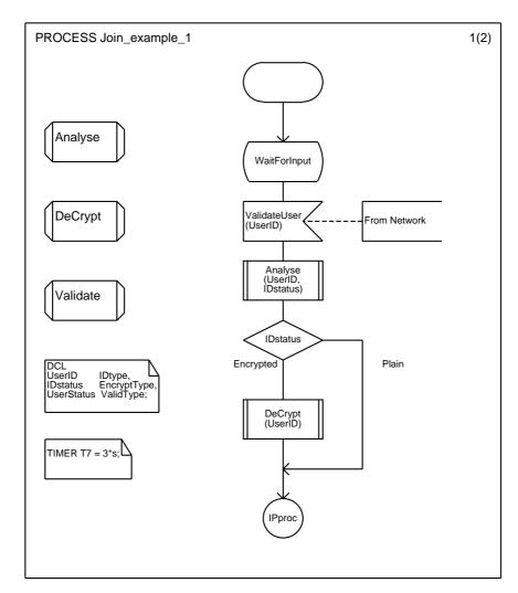
Figure 7: Paging using a connector symbol (page 1)
