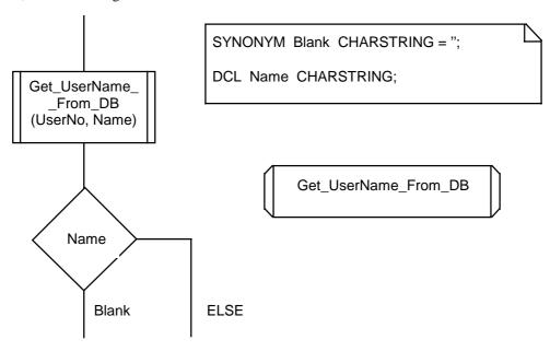
Figure 41: Decision based on a procedure's return parameter
