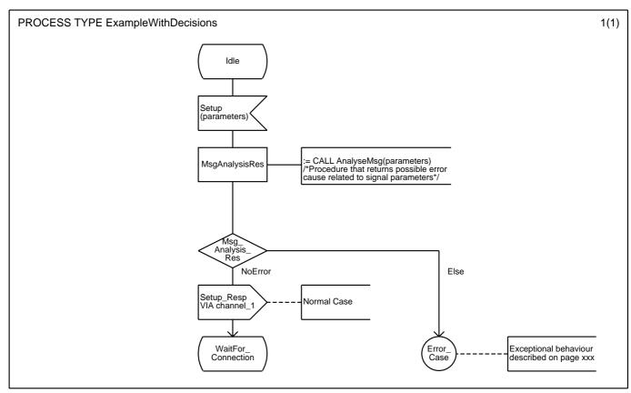
Figure 13: Part of process diagram showing only normal behaviour flow
