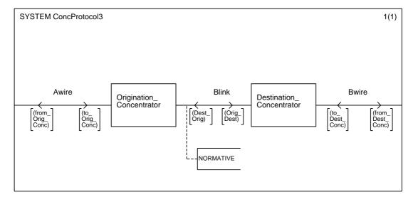
Figure 47: A minimal SDL model for the concentrator protocol standard example (distinct ends)
