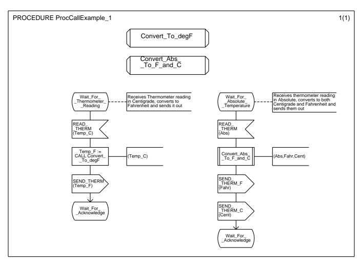
Figure 18: Examples of procedure calls
