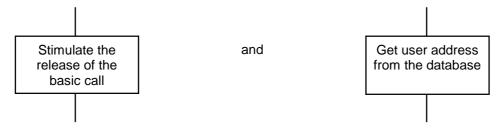
This notation is very easy to understand but it is not possible simulate or validate the action in the symbol. According to the strict definition of SDL, the text, "Stimulate the release of the basic call", is interpreted as a name at the start of an incomplete, and therefore incorrect, assignment statement. To make such expressions formal and executable, *convert informal text descriptions of actions into procedure calls and replace the task symbols with a procedure symbols*, thus:
