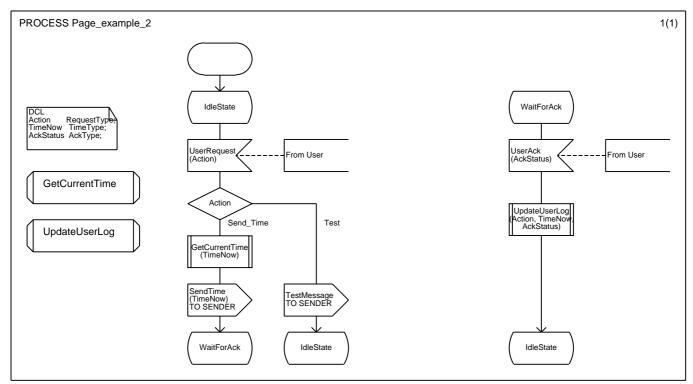
Figure 6: Transitions aligned on a single page
