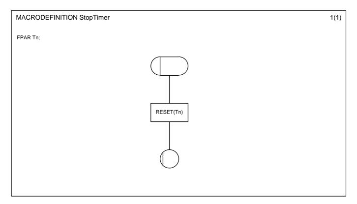
Figure 30: Macro definition for stopping a timer
