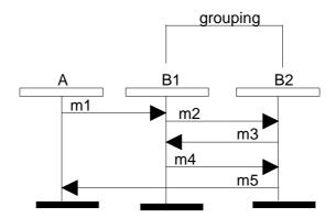
Figure 61: Suitable grouping and placement of strongly coupled instances
