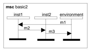
Figure 68: MSC containing an 'environmental' instance
