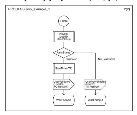
Figure 8: Paging using a connector symbol (page 2)
