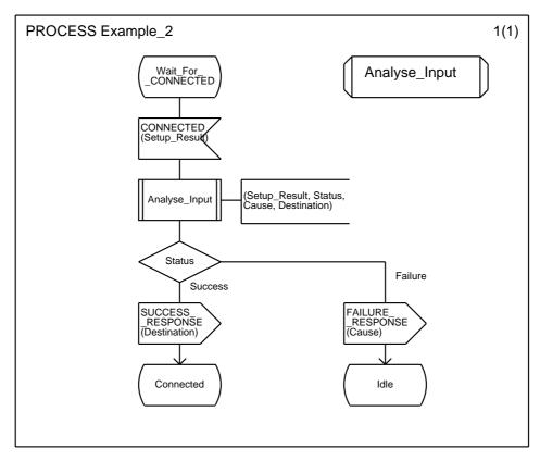
Figure 15: Message analysis example using a procedure
