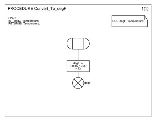
Figure 16: Example of a value-returning procedure
