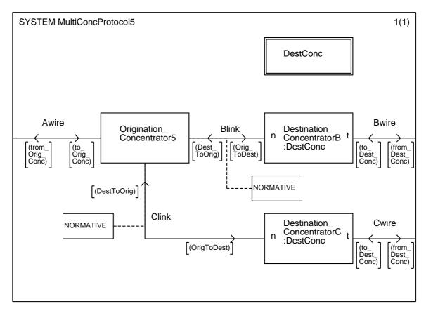
Figure 49: Static SDL model for a multi-link scenario.
