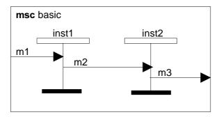
Figure 67: Complete MSC surrounded by an environment frame
