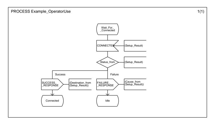
Figure 26: Examples of operator invocation
