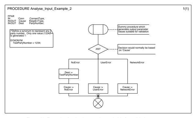
Figure 20: Example of a simple procedure suitable for validation purposes
