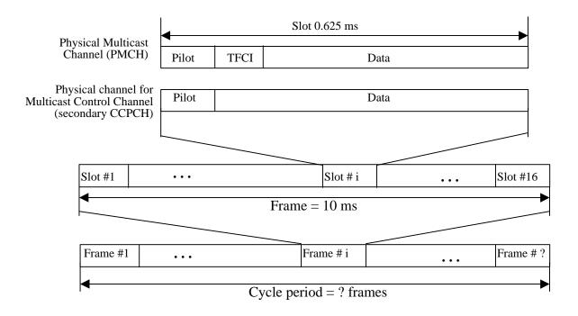
[Figure 3 Physical Channel Structure for multicast]
