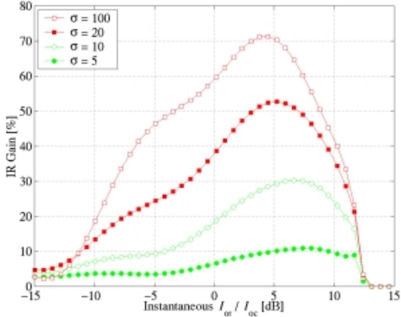
Figure 4: Achievable throughput gain with IR compared to Chase combining versus the instantaneous  $I_{or} / I_{oc}$  in dB. Results are shown for channel quality estimation errors  $\sigma$  of 5, 10, 20, and 100 dB.
