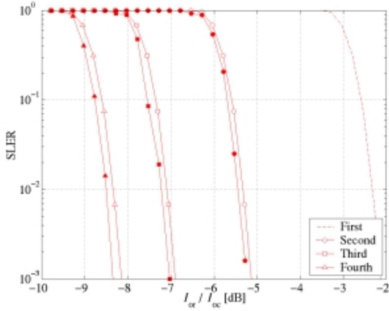
Figure 1: Simulated slot error rate versus  $I_{or} / I_{oc}$  in dB for MCS1 ( $K_{tot} = 3$ ). White and black markers are used for Chase combining and IR, respectively.
