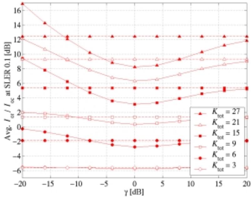
Figure 7: Average  $I_{or} / I_{oc}$  in dB that is required to obtain a slot error rate of 10% versus  $\gamma$  in dB.  $\gamma$  is the ratio of the received power in the original transmission and the retransmission. Results are shown for Chase combining(dashed lines) and IR (solid lines).
