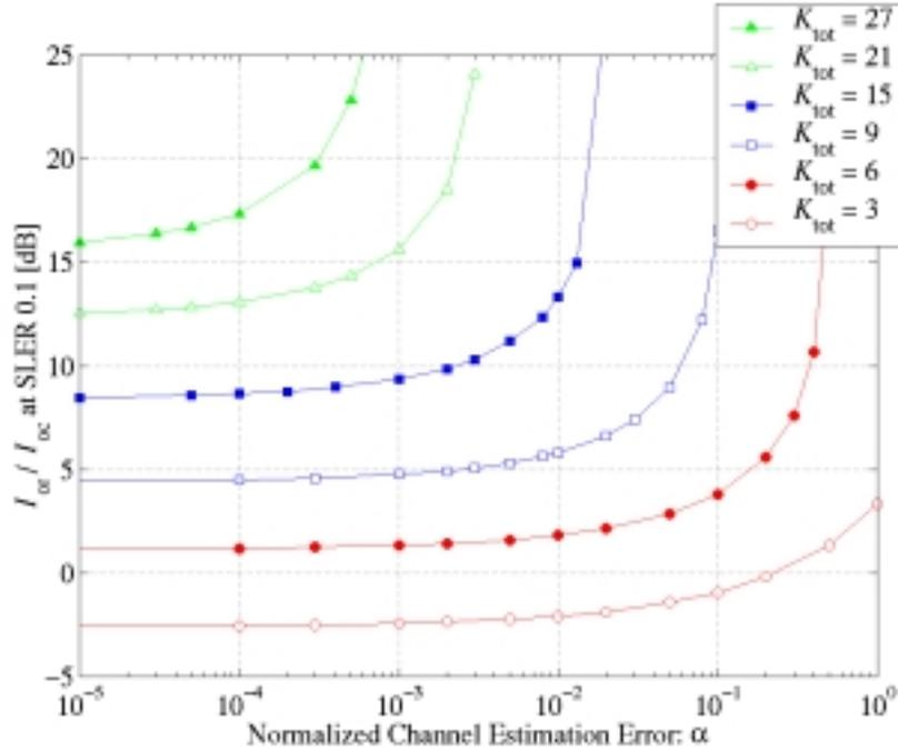
Figure 5: The required  $I_{or} / I_{oc}$  in dB to achieve a slot error rate of 10% versus the normalized channel estimation error  $\alpha = \sigma_e^2 / \sigma_h^2$ .
