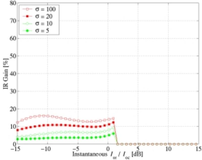
Figure 6: Achievable throughput gain with IR compared to Chase combining when using only MCS1-MCS3. Results are shown versus the instantaneous  $I_{or} / I_{oc}$  in dB for channel quality estimation errors  $\sigma$  of 5, 10, 20, and 100 dB.
