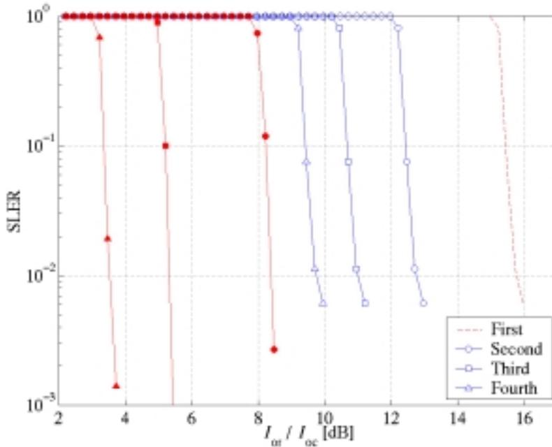
Figure 2: Simulated slot error rate versus  $I_{or} / I_{oc}$  in dB for MCS6 ( $K_{tot} = 27$ ). White and black markers are used for Chase combining and IR, respectively.
