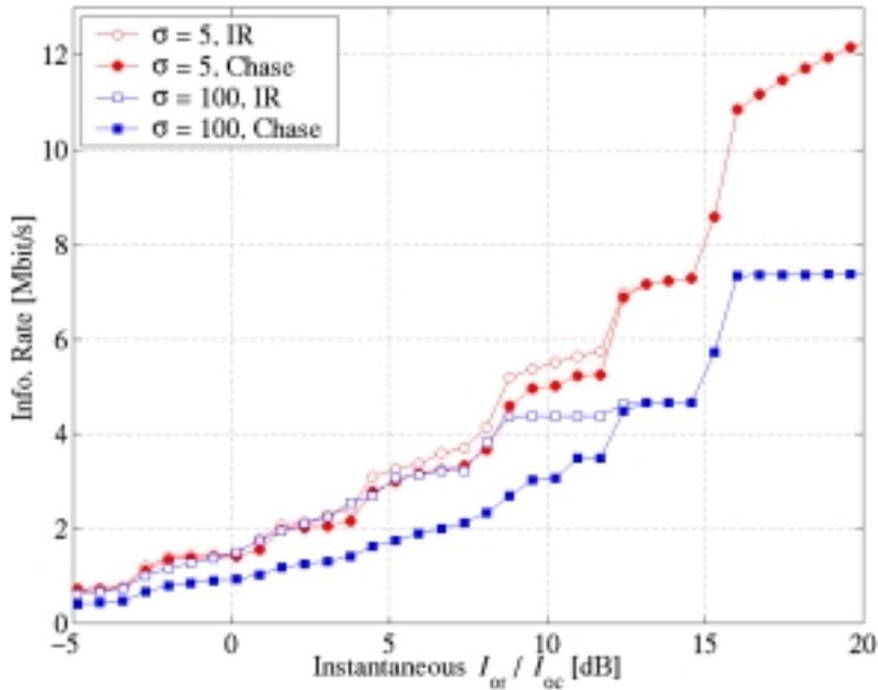
Figure 3: Throughput versus instantaneous  $I_{or} / I_{oc}$  in dB. The parameter  $\sigma$  is the standard deviation or the channel quality estimate error.
