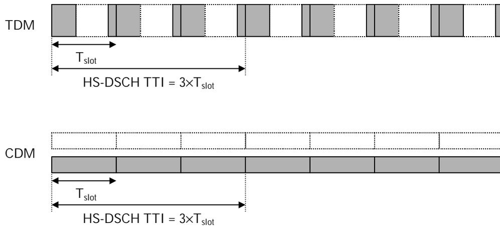
**Figure 3 Structure of uplink signalling when HS-DSCH data is not transmitted**
