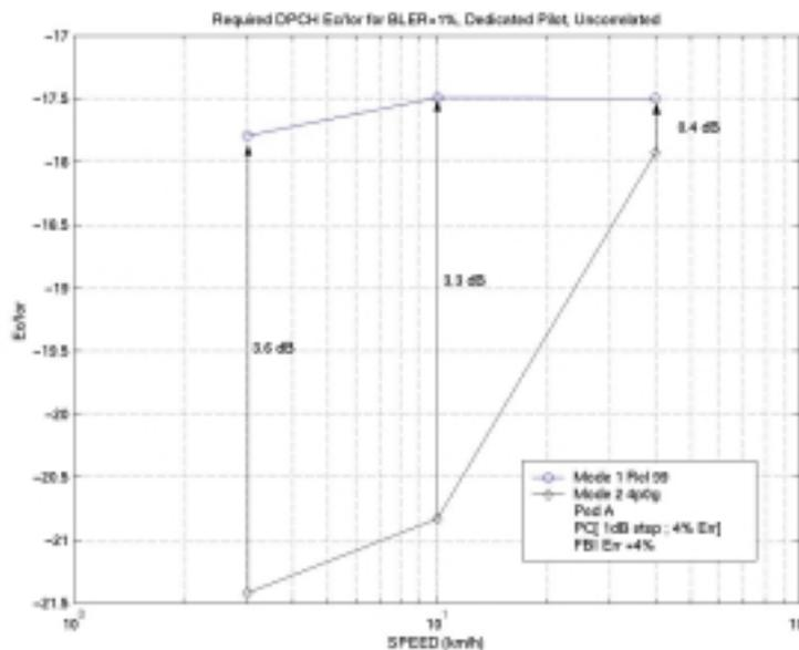
Figure 1 : 4-elements reduced state mode 2 for uncorrelated channel model
