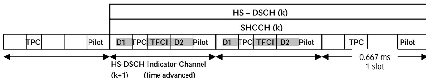
Figure 2. Timing of HS-DSCH, SHCCH, and time advanced HS-DSCH Indicator Channel. HS-DSCH Indicator (HI) Channel contains code space information for next HS-DSCH and SHCCH. In this case the HI Channel could be 2 (shown) or 3 slots like the HS-DSCH and SHCCH. A 3 slot HI channel requires less power.
