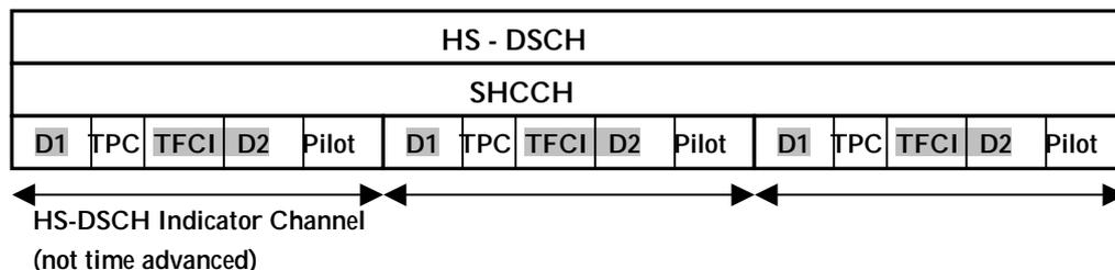
Figure 3. Timing of HS-DSCH, SHCCH, and HS-DSCH Indicator Channel when HS-DSCH Indicator Channel is not time advanced. TTI is 3 slots for all 3 channels and they are coincident such that all three would therefore be buffered and decoded at the same time. Information bits are in grey for current HI channel slots.
