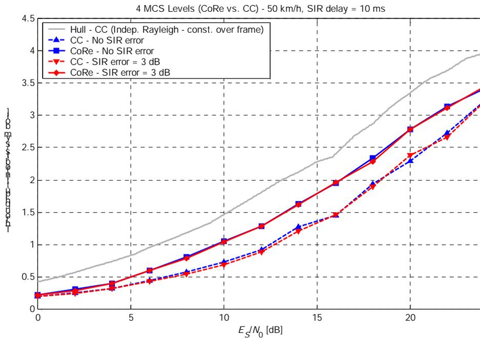
Figure 4. Throughput for 4 MCS levels, UE Speed = 50 km/h.
