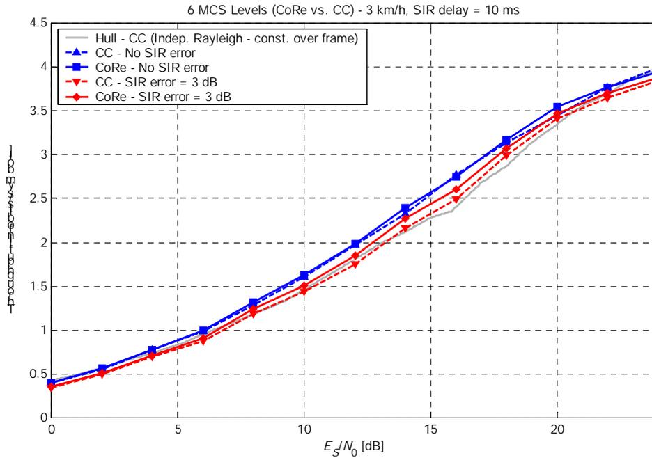
Figure 1. Throughput for 6 MCS levels, UE Speed = 3 km/h.
