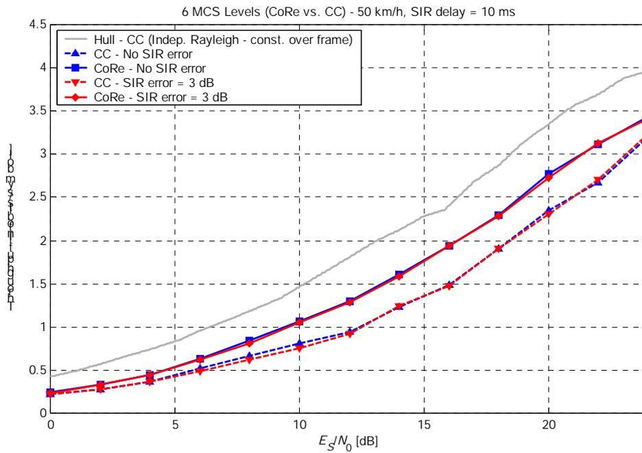
Figure 2. Throughput for 6 MCS levels, UE Speed = 50 km/h.
