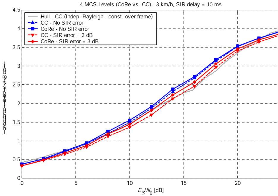
Figure 3. Throughput for 4 MCS levels, UE Speed = 3 km/h.
