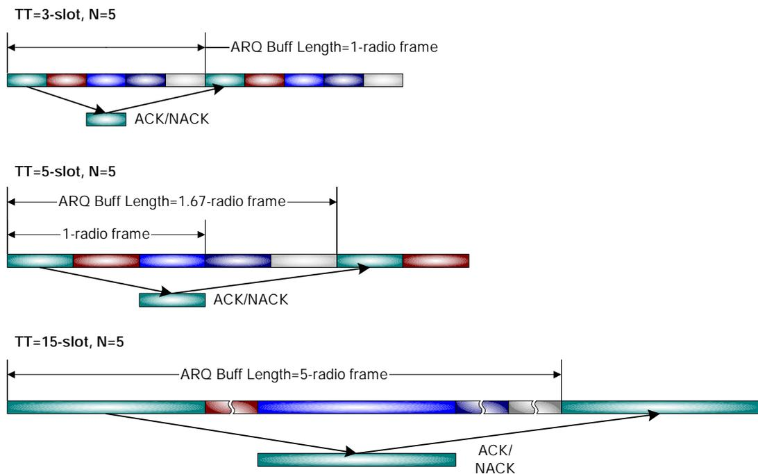
Figure 1 H-ARQ N-SAW channel structures with various TTI
