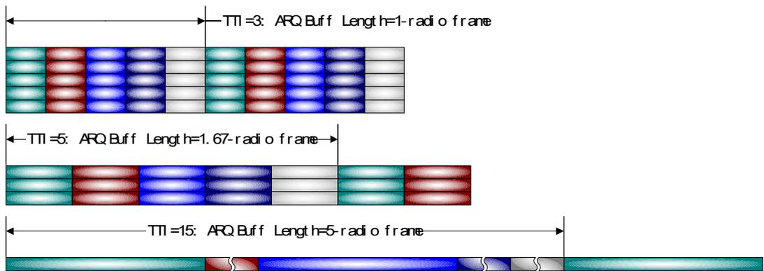
Figure 2 TTI dependent multi-code utilization
