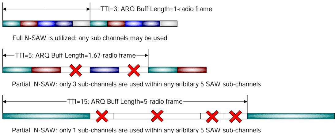
Figure 3 TTI dependent sub-channel utilization
