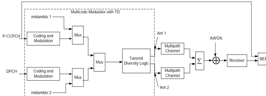
Figure 1. Simulation Testbench Block Diagram
