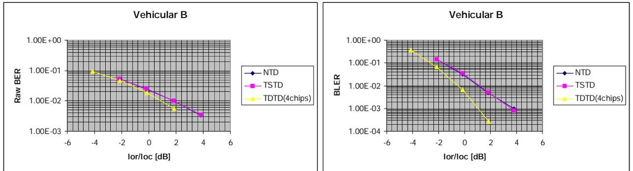
Figure 7. Raw BER and BLER for ITU Vehicular B case
