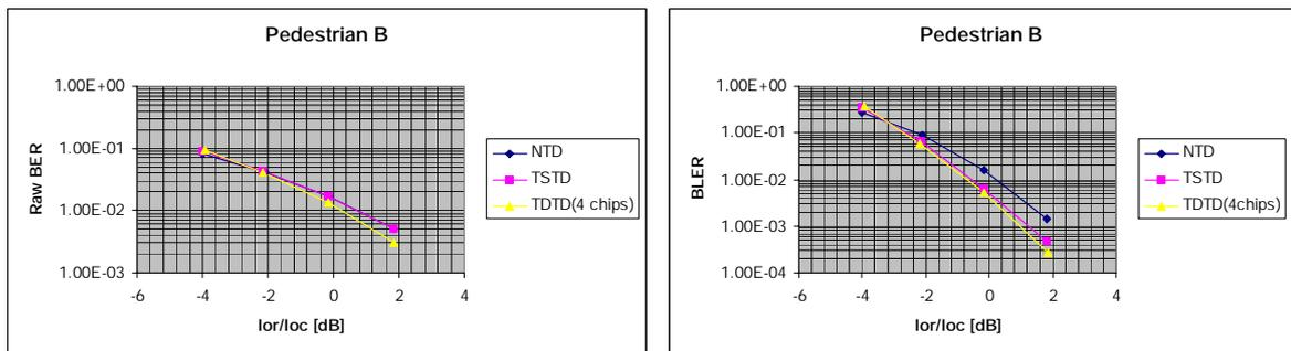
Figure 5. Raw BER and BLER for ITU Pedestrian B case
