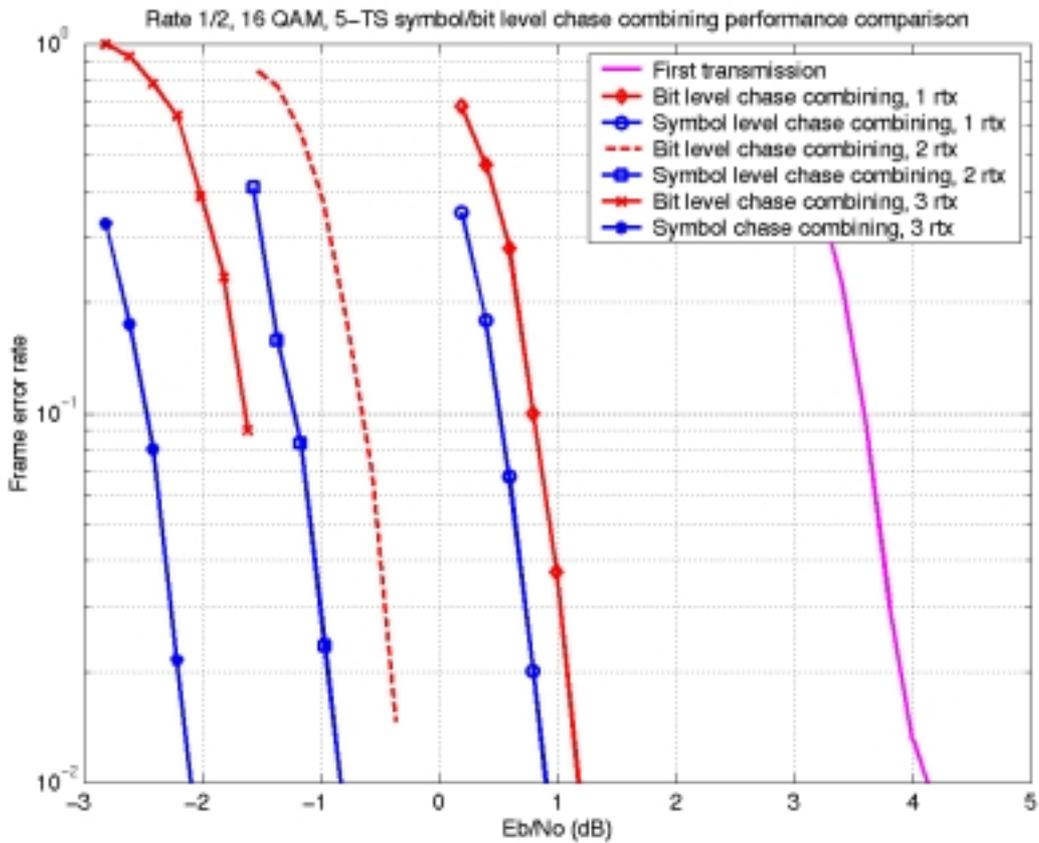
Figure 2: Performance comparison for bit level and symbol level Chase combining for AWGN, 16 QAM, rate 1/2, frame size 5-TS is shown.
