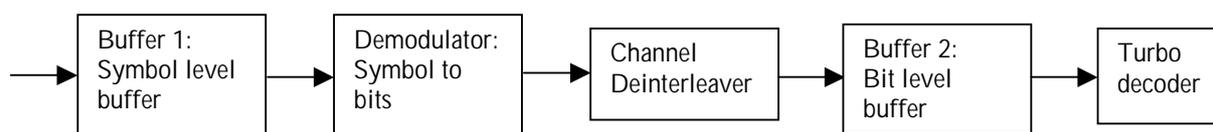
Figure 1: Block diagram of the receiver doing Chase combining is shown
