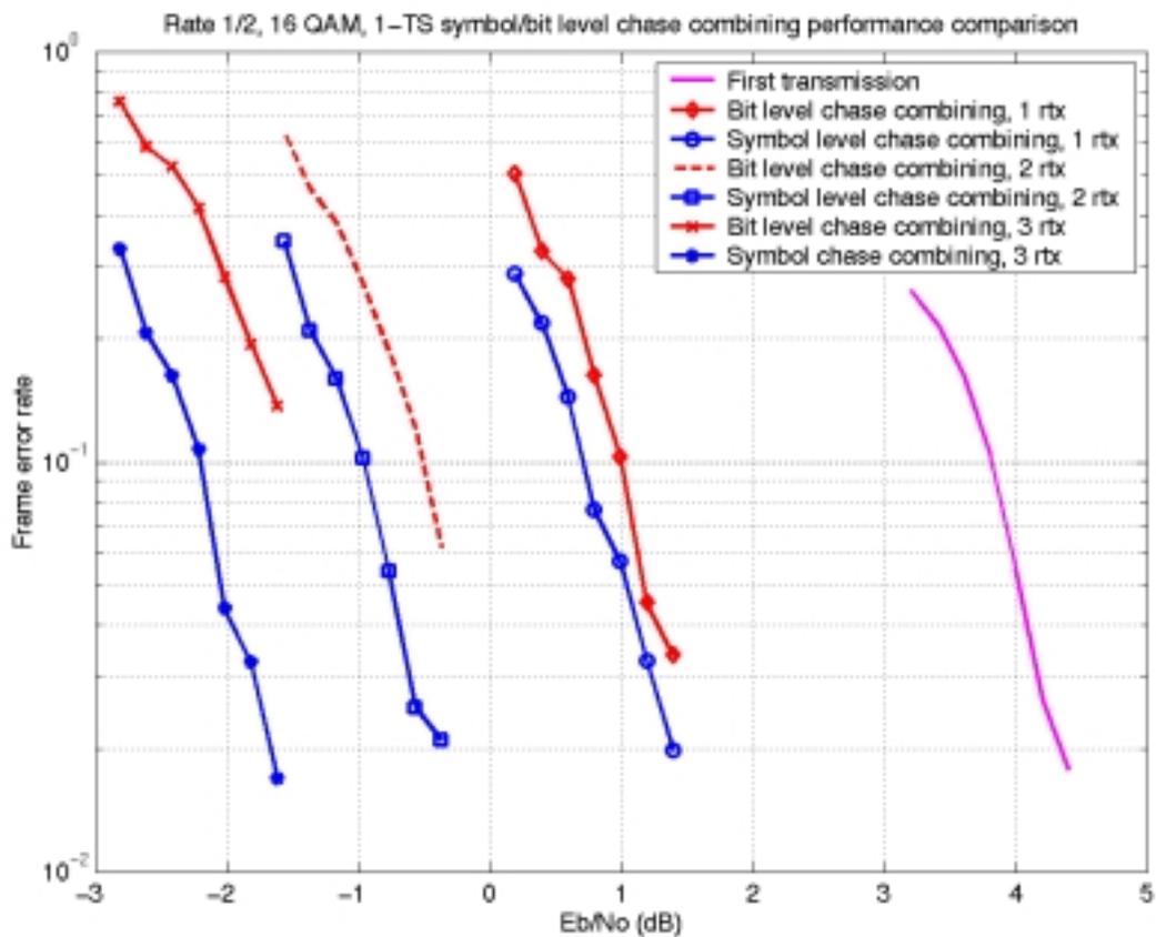
Figure 1: Performance comparison for bit level and symbol level Chase combining for AWGN, 16 QAM, rate 1/2, frame size 1-TS is shown.
