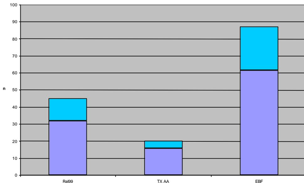
Figure 2: Comparison of cell capacity (in numbers of DPCH) between Rel99 mode 1, adaptive antennas without feedback and the eigenbeamformer
