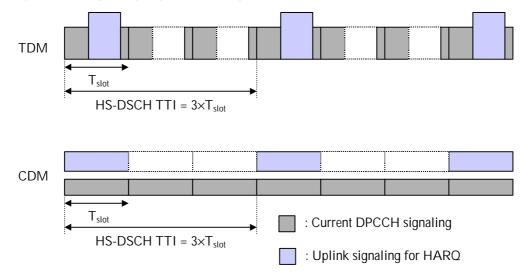
Figure 2 Structure of uplink signalling when HS-DSCH data is transmitted
