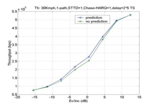
Figure 2. Throughput versus Ec/loc with and without channel prediction. Total delay=2 HSDPA frame, 1-path Rayleigh channel, speed = 30kmph, STTD on, HARQ with Chase Combining, ideal feedback. Max re-transmission=10.
