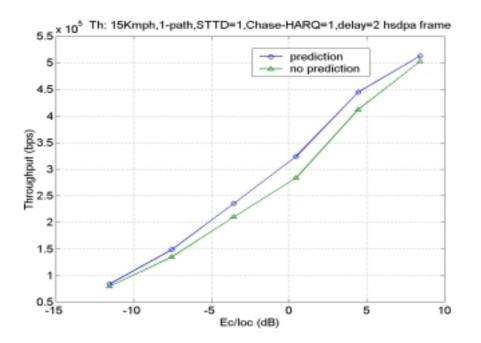
Figure 1. Throughput versus Ec/loc with and without channel prediction. Total delay=2 HSDPA frame, 1-path Rayleigh channel, speed = 15kmph, STTD on, HARQ with Chase Combining, ideal feedback. Max re-transmission=15.
