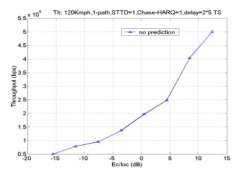
Figure 3. Throughput versus Ec/loc without prediction. Total delay=2 HSDPA frame, 1-path Rayleigh channel, speed = 120kmph, STTD on, HARQ with Chase Combining, ideal feedback. Max re-transmission=10.
