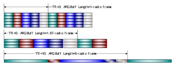
Figure 2 TTI dependent multi-code utilization
