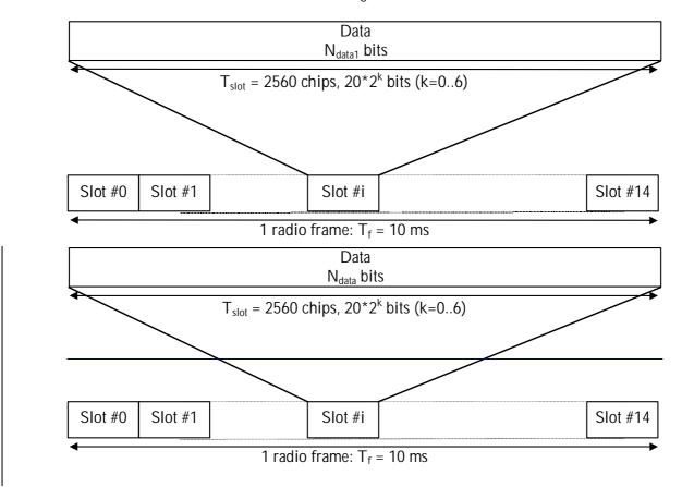
Figure 20: Frame structure for the PDSCH
