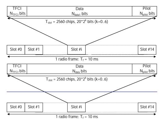
Figure 17: Frame structure for Secondary Common Control Physical Channel
