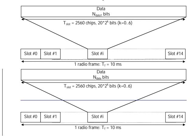
Figure 20: Frame structure for the PDSCH
